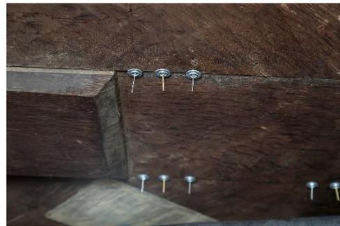
**Left:** One of the eight carbon plates on the calendar disk. Two groups of three wires each are visible. Each wire is passed through two drill holes and through gaps in the calendar disk. **Right:** On the rear side of the calendar disk, the wires go through buttons and are twisted to secure them in place. Both pictures by Edeltraut Altrichter / ITMZ.
